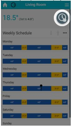
• Footprint mode: In this mode the system will heat the zone based on whether the zone is normally used at this time, and if there is anyone currently using the zone. The timer bars are not clickable in this mode as the schedule is automatically created by your Genius Hub.
