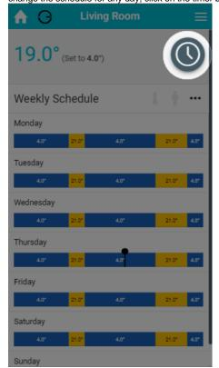
• Sense mode: Similar to Timer mode, the system will follow a chosen schedule, which you can edit at will. In Sense mode, you can also select periods to only heat up if there is occupancy detected during the selected times, to save from heating empty rooms.
