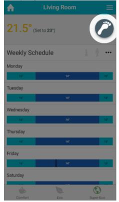
Override mode: This mode allows you to temporarily adjust the heating in the zone, by setting an override of a set temperature and duration. For On/Off zones, override switches the zone on for the duration set.
