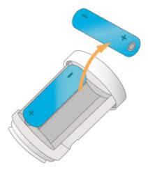
Put in the 2 new AA batteries, take note of the orientation shown on the screen.
