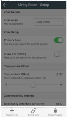
• Go to Zone Setup in the first zone again and assign the device which was in the second zone before the swap, but is now physically in the first zone.
