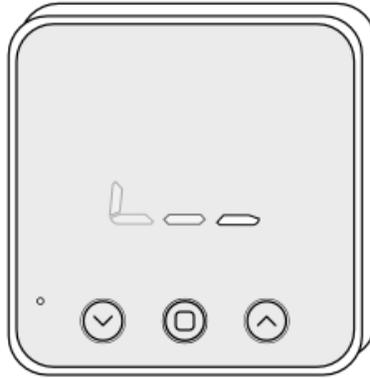
On success, the Room Thermostat will show 'INC' and will have been assigned a number, write this number on the side of the device.
