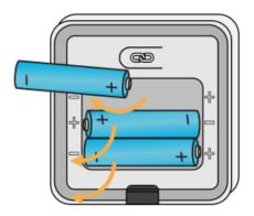
Put in the 3 x new AA batteries.
