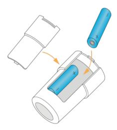
Replace the battery cover, starting at the top (nearest the screen). Now the hub needs to get ready to add the device.
