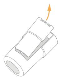
Ensure there are new batteries in the Genius Radiator Valve and they are correctly oriented.
