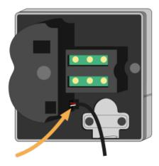
6. Re-fasten the Electric Switch, re-attach the cover (starting at the top) and power on the Hot Water Time & Temperature addon. Now select the Electric Switch on the app. The ID of the Electric Switch may be printed on a sticker on the button of the Electric Switch.
