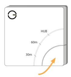
3. Remove the cover from the Electric Switch.
