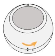
Pull the back of the Motion Sensor away from the body, you may find a thin, flat screwdriver helps to separate the two halves.
