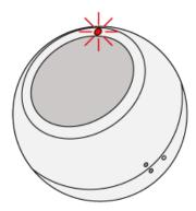
In Security Mode, the Genius Motion Sensor will flash each time it detects occupancy in 30 second intervals. As this increase in action causes the battery to drain more quickly and customers an find it distracting, this mode can be toggled between.
