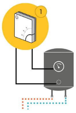
This is where you have temperature control from the app, and the hot water is controlled by an Electric Switch with a Temperature Probe next to the hot water tank which controls an electric element element inside the tank.
