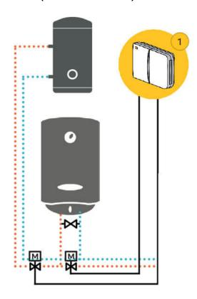
This is where you have on/off control from the app, and the hot water is controlled by a Dual Channel Receiver which controls zone valves near the boiler.
