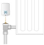
6. Press and hold the button for 3 seconds until the valve starts to buzz and a temperature appears on the screen. This takes the valve out of Mount Mode.
