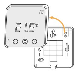
2. Turn the Room Thermostat over, so the screen is facing away from you and pull out the plastic tab to connect the battery.
