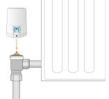
6. Press and hold the button for 3 seconds until the valve starts to buzz and a temperature appears on the screen. This takes the valve out of Mount Mode.
