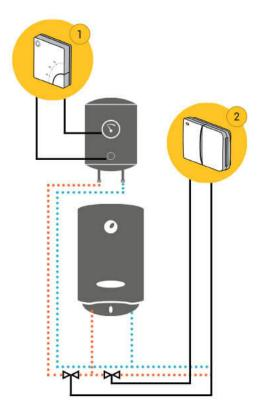
This is where you have temperature control from the app, and the hot water is controlled by a Dual Channel Receiver which controls zone valves near the boiler, and there is an Electric Switch with a Temperature Probe next to the hot water tank.
