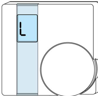
After 10 seconds the screen shows 'LP' when the device has included successfully. If 'LP' is not displayed this is not a problem so long as a number for the device is included successfully in the status box below.
