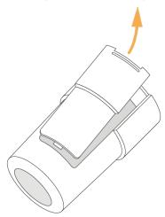
Once you have completed your work, replace the battery and the plunger will retract and the Genius Radiator Valve will start to communicate with the Genius Hub once more.
