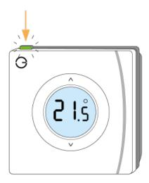
The green light will stop flashing when the device has included successfully.
