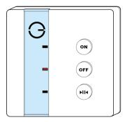
On success, the Single Channel Receiver has been assigned a number, write this number on the side of the device.
