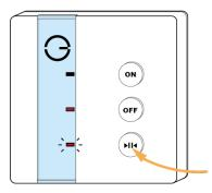
The bottom red light stops flashing and the top green light will flash briefly. The 'Off" light turns red when the device has included successfully.
