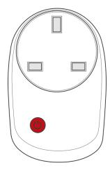
**d.** A Powered Room Thermostat shows a **red** light to the bottom right of the display.
