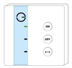
b. Hold down the Hot Water button on the the Dual Channel Receiver (the light at the top-left with turn green for 2 seconds).
