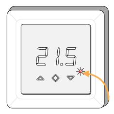
e. An Electric Relay shows a red light behind the button on the device. You will need to remove the blanking front plate to see this.
