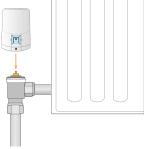
6. Press and hold the button for 3 seconds until the valve starts to buzz and a temperature appears on the screen. This takes the valve out of Mount Mode.
