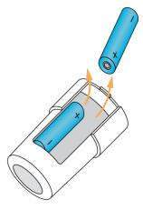
Put in the 2 new AA batteries, take note of the orientation shown on the screen.
