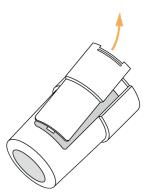
Remove the 2 x AA batteries, (note the orientation of the batteries, one is up and one is down).
