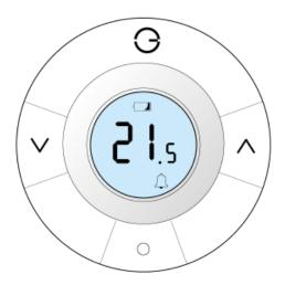
The batteries are low in the Genius Radiator Valve and they will probably only last for another few weeks before the valve stops working altogether.
