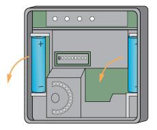
Put in the 2 new AAA batteries, (note the orientation of the batteries, both have the positive at the top).
