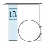
The batteries are low in the Wireless Room Thermostat and they will probably only last for another few weeks before the thermostat stops working altogether.
