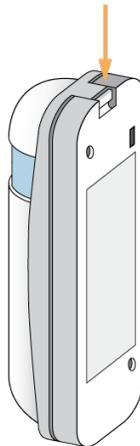
Ensure there is a working battery in the Room Sensor and it is correctly oriented.
