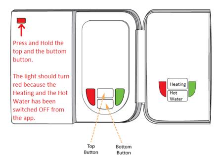
• Go to the Device list on the app and check if the traffic lights of the Dual Channel Receiver are red.
