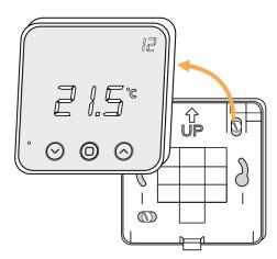
2. Turn the Room Thermostat over, so the screen is facing away from you and pull out the plastic tab to connect the battery.
