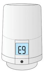
The Genius Radiator Valve shows the 'E9' 'Valve closing error' if it tries to close the flow of water through the radiator a number of times and fails. Unmount and remount the Genius Radiator Valve to see if this fixes the problem.
