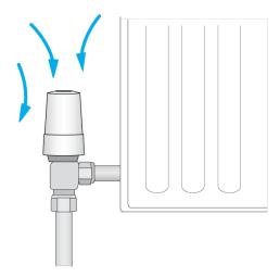
The Genius Radiator Valve features an 'open-window' function, which closes the valve if the room temperature is falling dramatically, thus reducing the wasted heat if the app is set to heat a room but a window is then opened.
