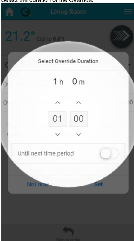
**i** Instead of choosing a duration, it is possible to override until the next duration. This is often used to bring the heating on earlier than usual as if the same temperature is chosen the system will move from the Override to the Timer period seamlessly.
