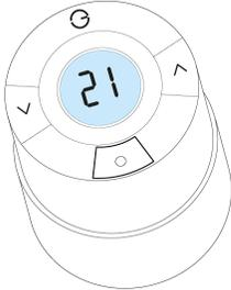
Each Radiator Valve comes with two adaptors. The two adaptors fit the Radiator Valve onto either an M30x1.5mm thread (the UK standard which fits most brands of TRV) or a Danfoss RA fitting (the adaptor with the grub screw). To mount the Radiator Valve:
