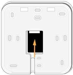
3. Plug the USB power cable, both to the Genius Hub (until you hear it click) and into the power supply provided, and plug into a wall socket. A green light will appear on the left hand side.
