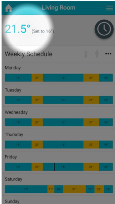
1. **The measured temperature:** This is the current temperature in the zone, and is displayed if the zone has a device which feeds the temperature back to the app (such as a Room Sensor or Thermostat).
